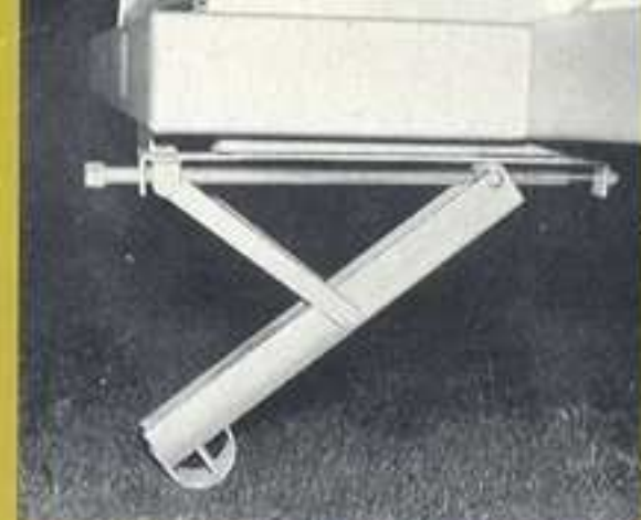
Stabilizing jacks standard on Continental models. Optional on other models.
