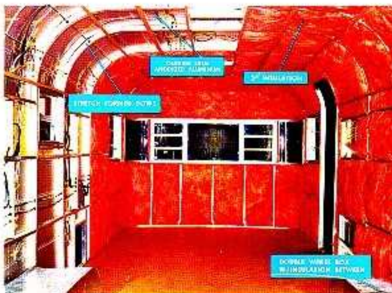
The body of your Silver Streak trailer is two complete shells one inside the other, separated by a blanket of 2 inch high density fiberglass insulation in roof and sidewalls riveted together as one unit on extruded aluminum stretch formed bows and stringers. Outside skin is of .032 anodized aluminum. Inside skin is .092 vinyl aluminum. A plastic vapor barrier is placed on all cross members and ribs to prevent "sweating." Double wheel well covers with 2 inch fiberglass insulation.
