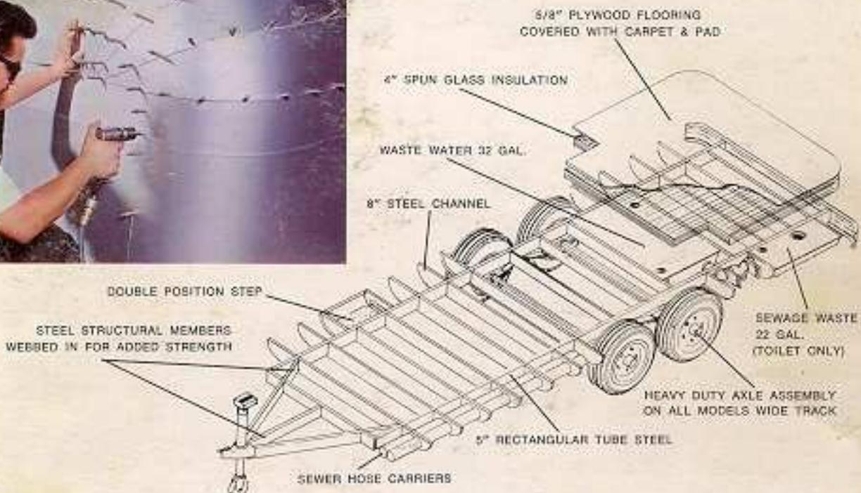
Underbelly is completely sealed for frame protection and prevents dust and the elements from penetrating the interior.
