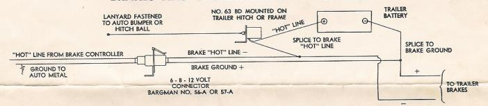
**INSTALLATION IS SIMPLE:** Mount 63 BD on hitch of trailer with one screw in mounting bracket. Position bracket so there is no strain on lanyard between trailer and tow car. Install storage battery in trailer and connect wires as shown in schematic wiring diagram above.
