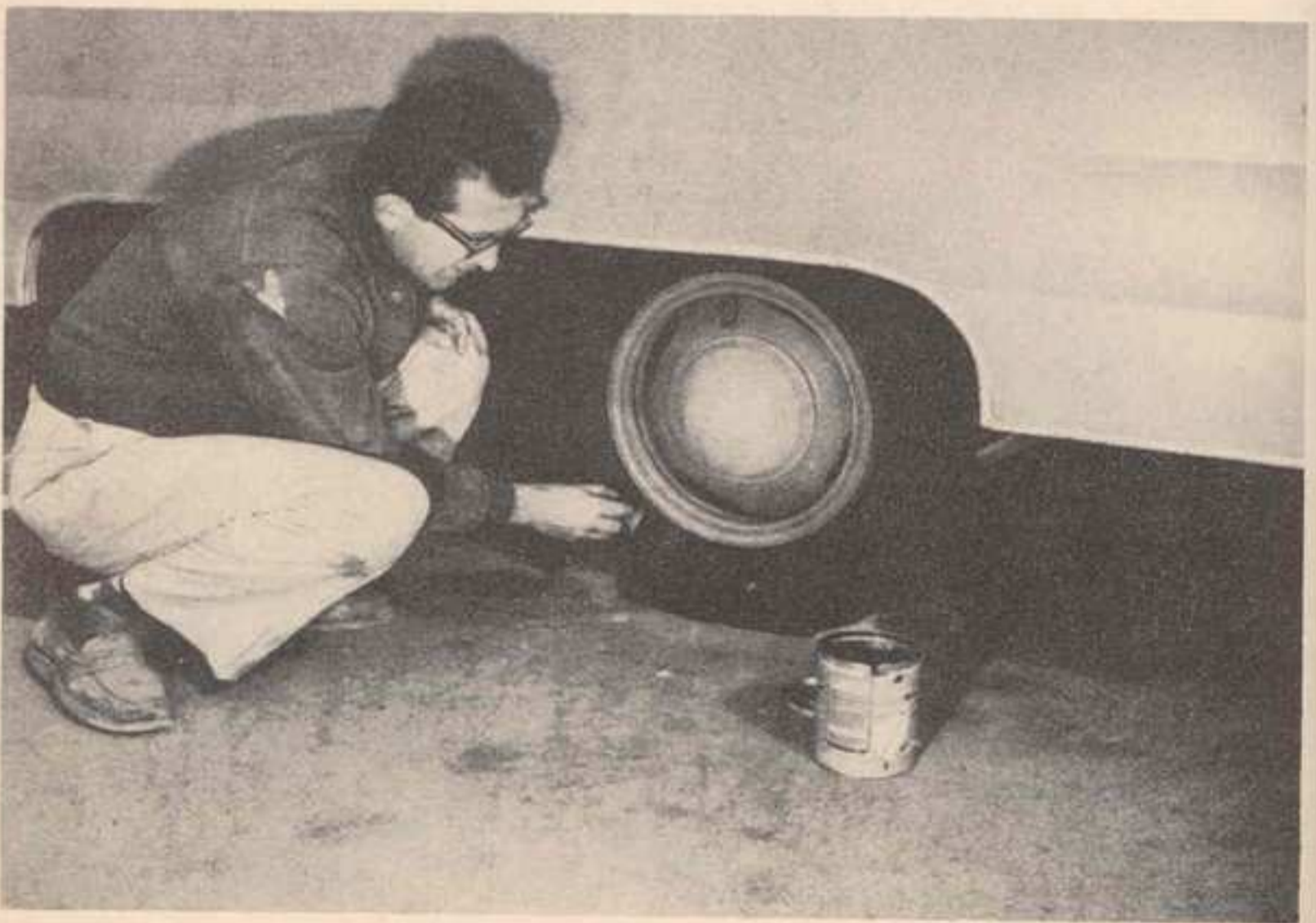
Keep tires on parked mobile homes painted with synthetic rubber protective paint.
