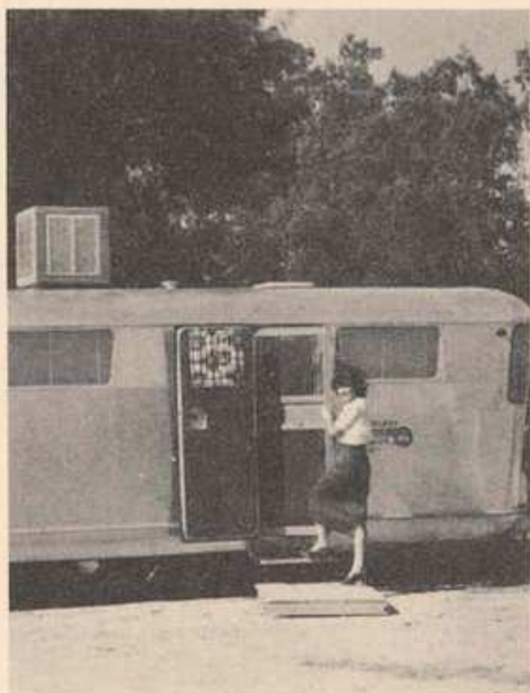
Courtesy International Metal Products Co. Evaporative coolers are frequently installed on roof over a ventilator opening from which vent top has been removed.
