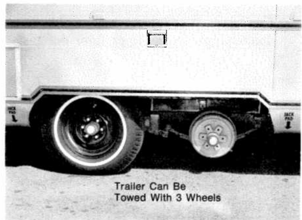
Figure 5 Trailer Can Be Towed With 3 Wheels
