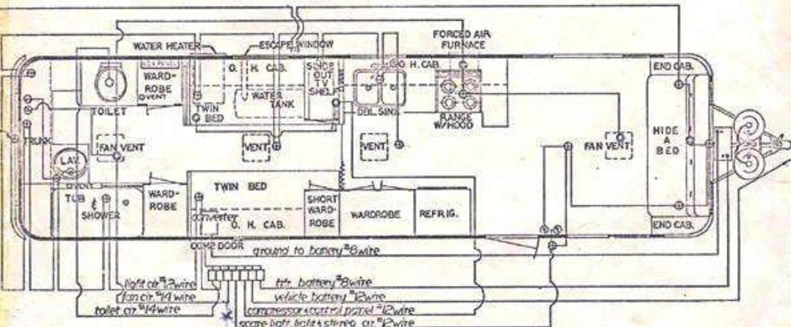
battery circuits shall be separated from other circuits and shall be protected per combustible material per
